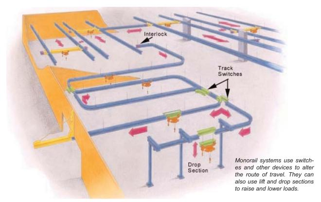
Automation can be as basic as simply picking up and delivering loads without operator assistance. An automatic monorail can also be programmed to raise, lower, and rotate the load; automatically store finished or semi-finished goods; or route coded products to appropriate points on the assembly line. Automatic Monorail Systems have been built with multiple routes and multiple elevations. The variations are endless.
