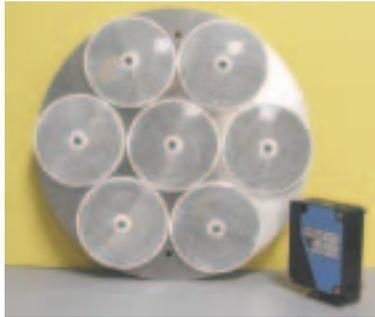
**LED Photoelectric Sensor Kit for On/Off Switching.** Recommended for End Collision Avoidance Detection. Includes Mounting Bracket, Reflector Array and Hardware Sensor. Relays can open or close a circuit. For use with 24 to 240 VAC or 12 to 240 VDC outputs for N.O. or N.C. Circuit Control operating distance range from 3 to 45 feet.
