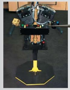
The engine-handling device shown uses the unique features of the InteLIFT balancer. Features include: auto clamp, interlock, up control disable, weight sensing with automatic alarm, and keyed lockout.
