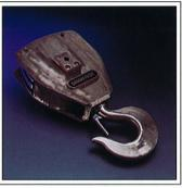
Bronze Hooks & Lower Blocks Solid, cast bronze hooks reduce the possibility of sparking in the event the hook strikes steel or other ferrou metal objects. Hooks are provided with stainless steel, spring-loaded safety latches as a standard feature The entire lower block body is fabricated from solid bronze plate. Solid bronze is used instead of coated steel because coating can chip or wear off - solid bronze does not
