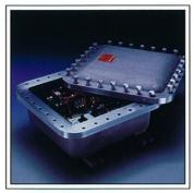
Nema 7/9 Control Enclosures Nema control enclosures are designed to reduce or eliminate the risk of explosion in hazardous environ ments. Nema 7 enclosures prevent ignition of gas external to the enclosure by containing the explosion within the panel. Nema 9 enclosures are sealed to prevent an explosion by excluding the entry of explosive amounts of hazardous dust
