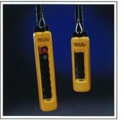
Intrinsically Safe Controls & Pendants Intrinsically safe systems engage a motion's contactors with electrical components operating at voltages too low to cause ignition of gasses or dusts. While the motion's controls must be housed in a Nema 7 or 9 enclosure, the pendant station can use a smaller, lighter, standard enclosure (as shown) reducing operator fatigue and permitting easier operation of the equipment.
