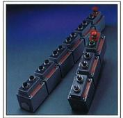
Nema 7/9 Pendant Stations Nema 7/9 pendant stations use standard control components in an explosion proof enclosure to prevent ignition of explosive materials outside the pendant station. The enclosure prevents ignitable dust from seeping in, and contains any
