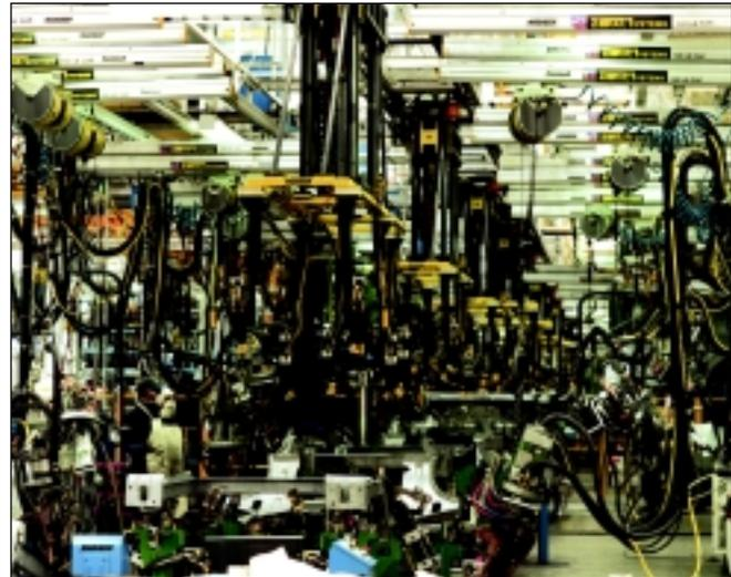
IR Zimmerman bridge and runway system in a manufacturing plant.
