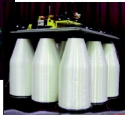
*The spool handling device shown here used by a major pharmaceutical products manufacturer, has Dual Controls. The spools are stacked 3-high in a box and the Dual Controls enable the operator to pick up spools without bending.*
