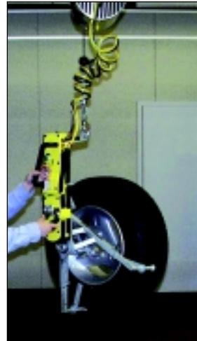
*Tire handling device with 90 degree manual rotate.*
