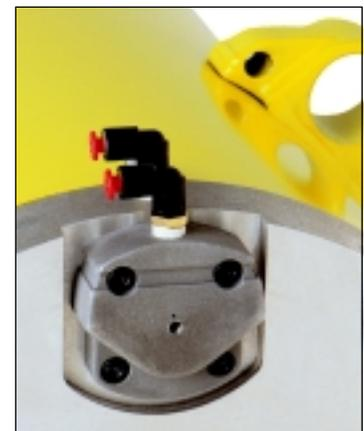
**Z Stop:** The optional Z Stop is a patent pending device that will eliminate the down-drift of suspended loads or tools during shut down or at night when the air supply is shut off. The Z Stop will stop drift within 6 inches (152.4 mm) and put the Balance Air into a mechanically locked position preventing damage to tools or objects below the suspended load. Available for use on all 10 inch (254 mm) diameter units.
