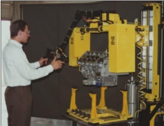
*Air clamp handling device for engine rollover*
