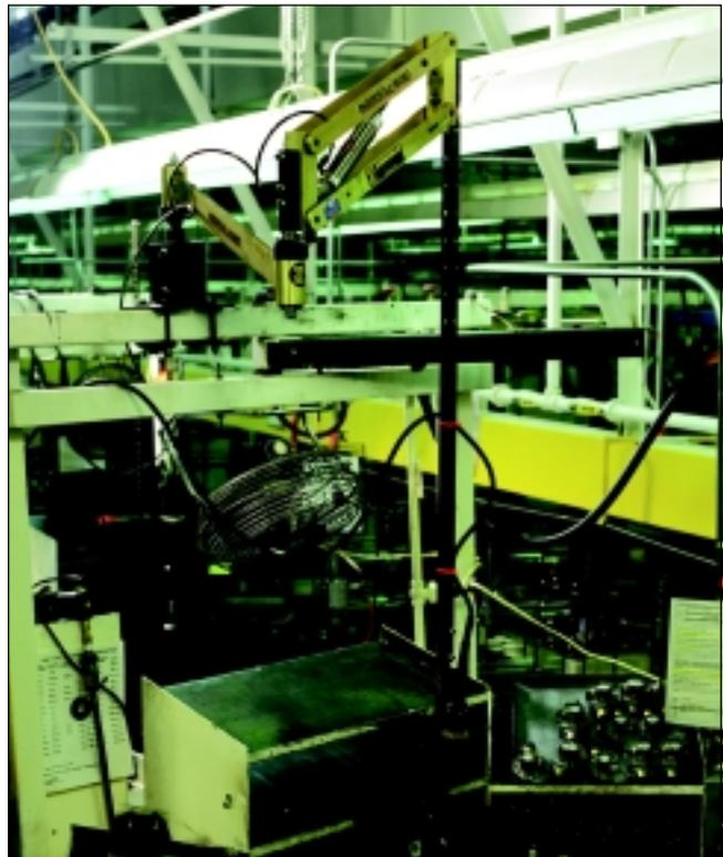
*EZ Tool Arm in an assembly process*
